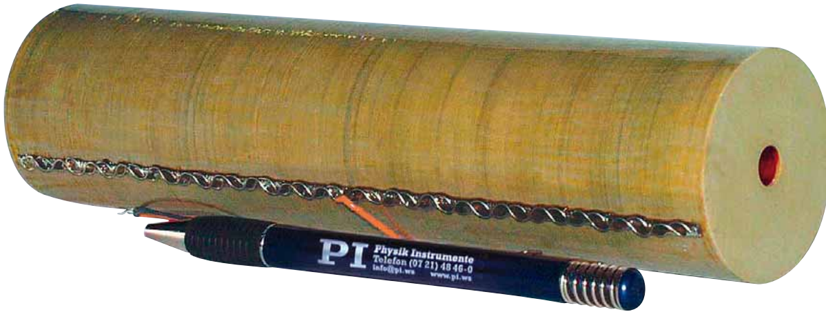
Custom PICA™ Thru piezo actuator with 56 mm outside diameter, 8 mm inner diameter, 250 \mu m displacement. Pen for size comparison
